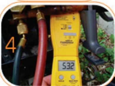
4: Measure suction line temperature near suction service valve. 53 degrees
